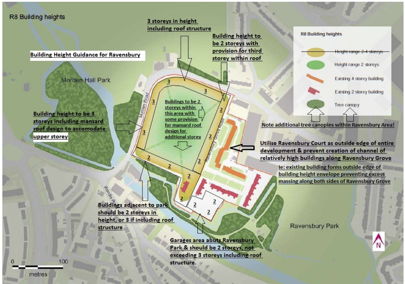
Image above: annotated R8 Building Heights map with guidance on heights proposed
