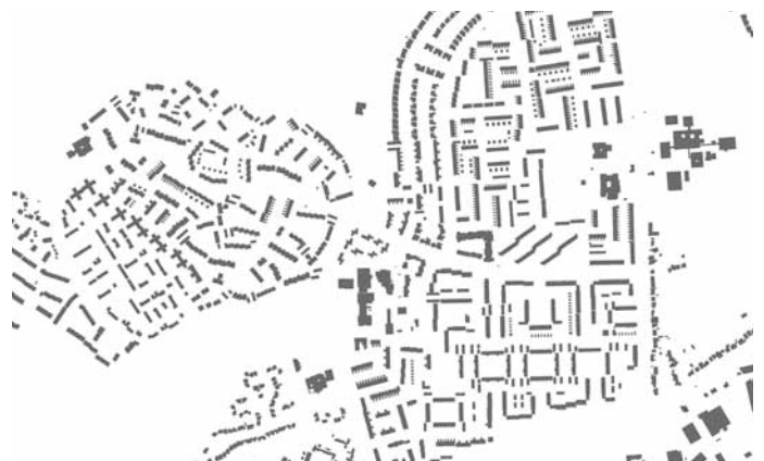
Above: A 'Radburn' layout in Grove Hill, Hemel Hempstead, with segregated routes and a confused building arrangement.
