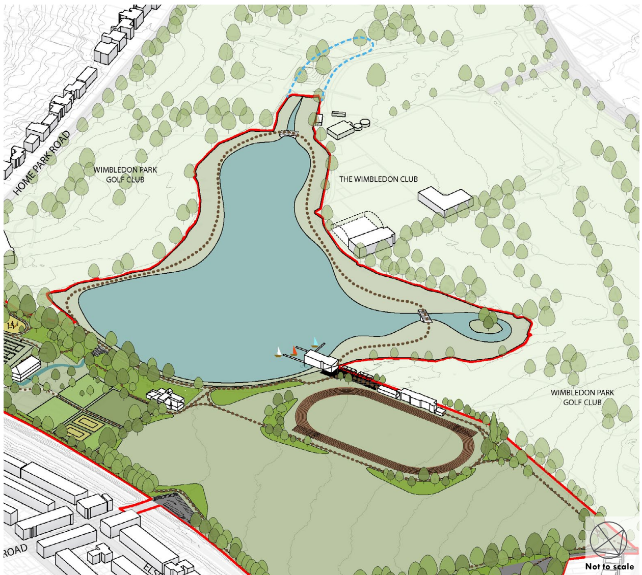
Fig. 5.9 Extract from the proposed masterplan with existing Lake outline shown in red, and proposed new lake outline with new perimeter path as a dotted brown line.
