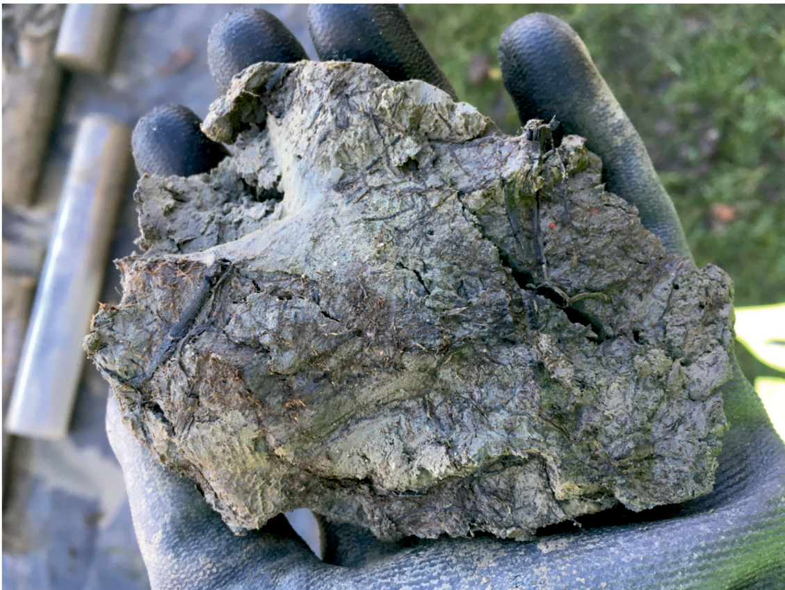
Fig 4 Photograph showing unidentifiable organics and CBM flecks in redeposited London Clay (WBD19_WS03)
