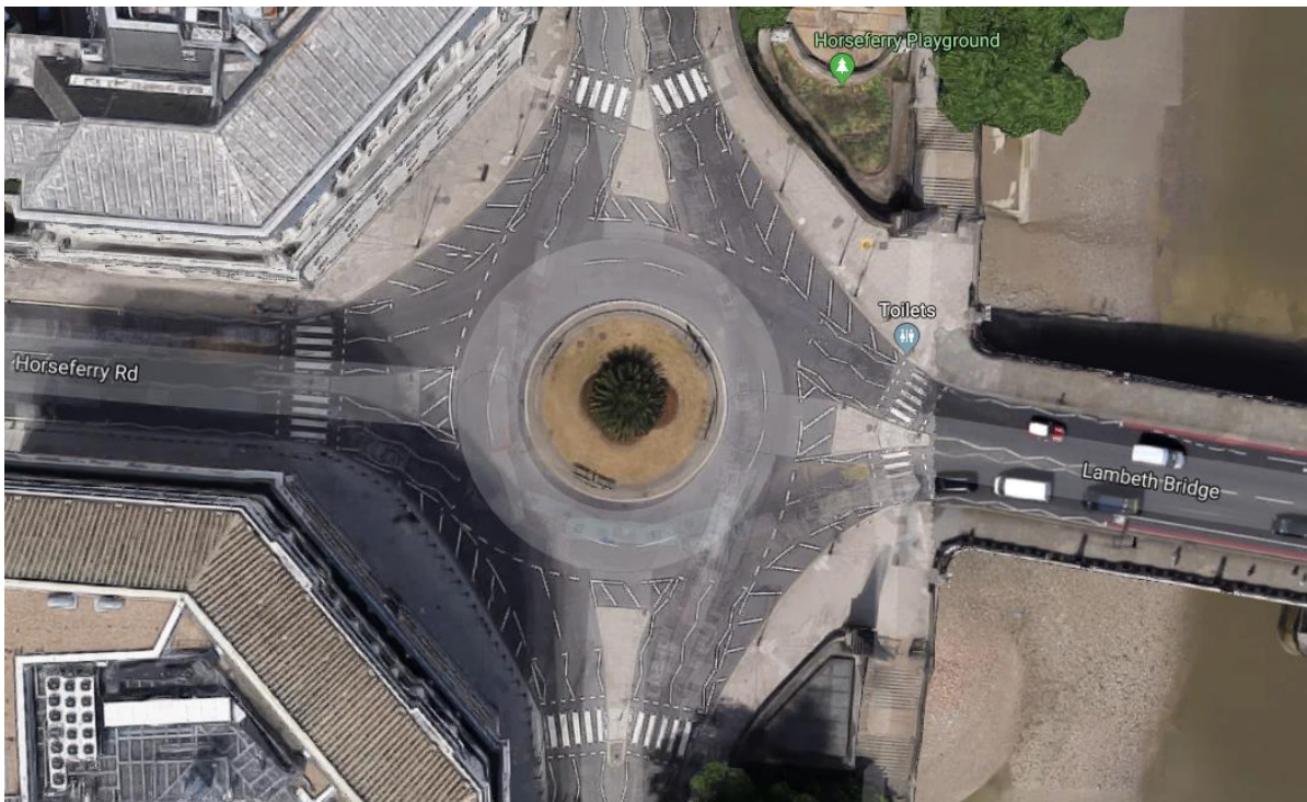
Figure 8: Horseferry Rd/Lambeth Bridge Roundabout, London. Zebra crossing on each arm.
