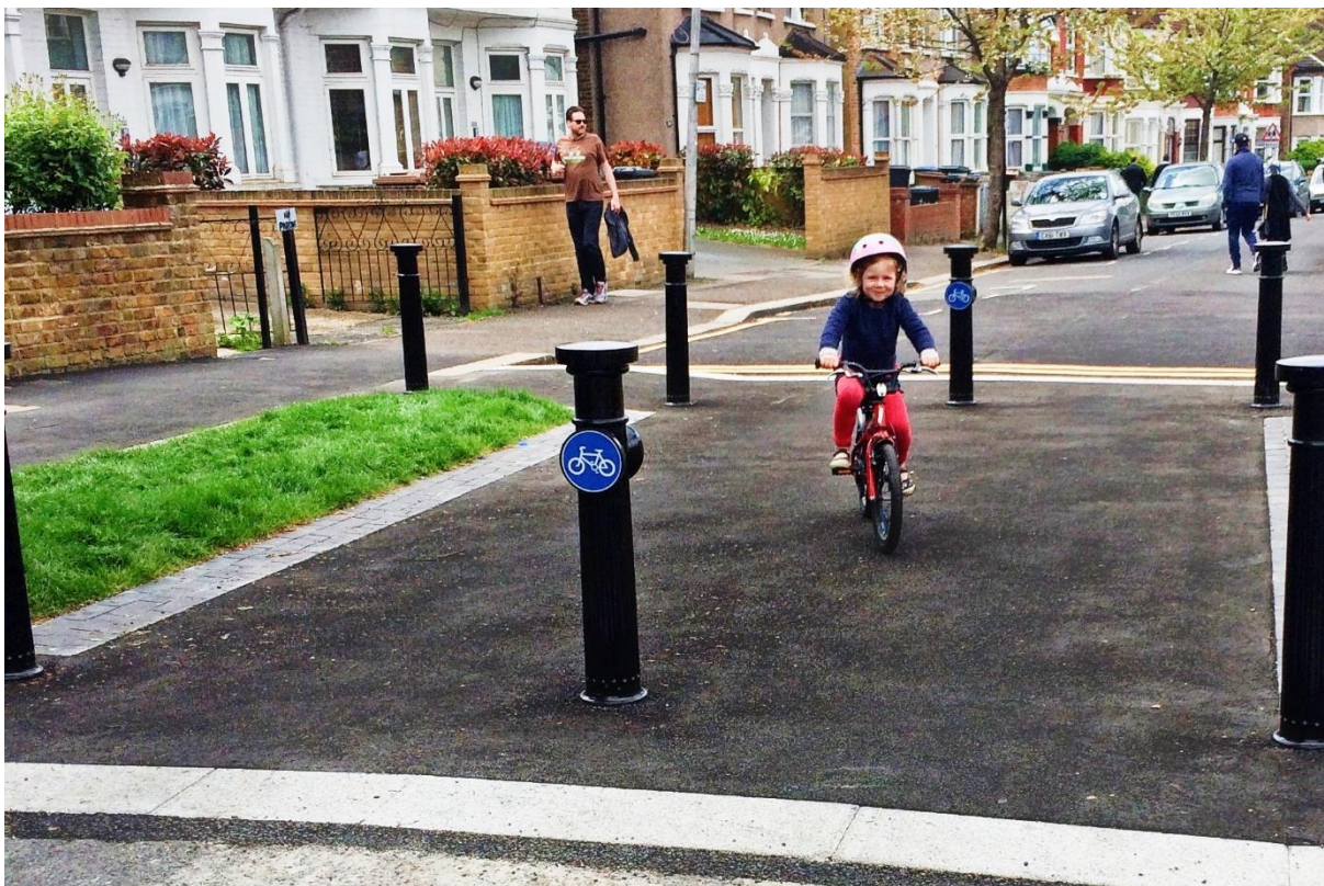
Figure 18: Modal filter. Cheap and effective. Can easily be trialled on a 12-month basis to see how residents take to it. Sheffield example
