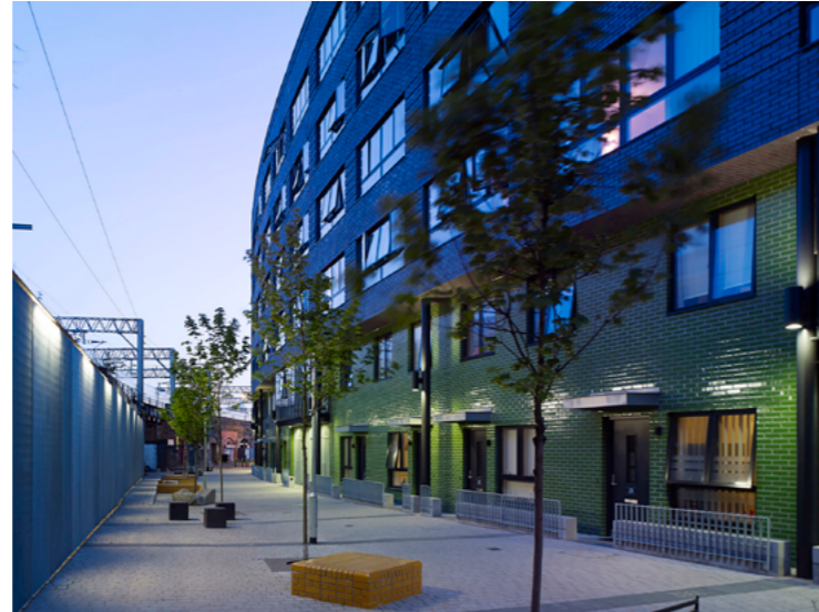
Fig.7.25 - The new homes provide a dual aspect with living rooms and kitchens facing the busy railway line opposite. This helps position bedrooms on the quieter side of the building. (Mint Street Housing, Tower Hamlets by Pitman Tozer Architects) [Credit: Kilian O'Sullivan]
