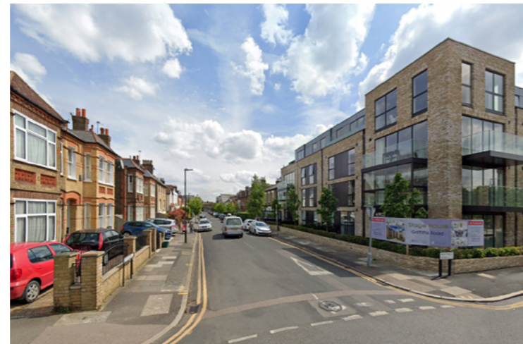
Fig.5.5 - Taller building in residential context. The proposal steps up to four storeys in a predominately 2 storey neighbourhood. The use of a set back fourth floor, contrasting material pallet and landscaping are used to minimise its impact on the street scene. (Griffiths Road, Wimbledon by 3W Architects)
