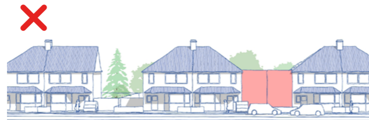
Fig.5.7 - Maintaining rhythm Conjoining buildings can create long street frontages and have a negative impact on the character of the street.
