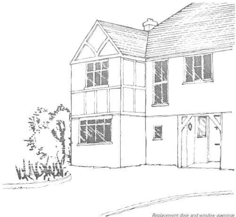
Replacement door and window openings
