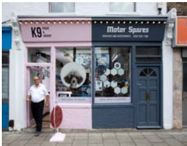
Pride and Groom and Motor Spares in Nunhead share the same shop front. 2 shops sharing the same premises can still have their own identity and branding. The width of the sign matches the width of the shop front. Architectural features like pilasters and corbels frame the shop front and unify the shop. Festoon lights illuminate the fascia sign at night, but they also give the shop a distinct appearance.
