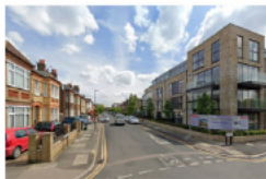
Fig 5.9 - Taller building in residential context. The proposal steps up to four stories in a predominantly 2 story neighbourhood. The use of a set back fourth floor, contrasting material palette and landscaping are used to minimise its impact on the street scene. (Driffell Road, Wimbledon by JW Architects)
