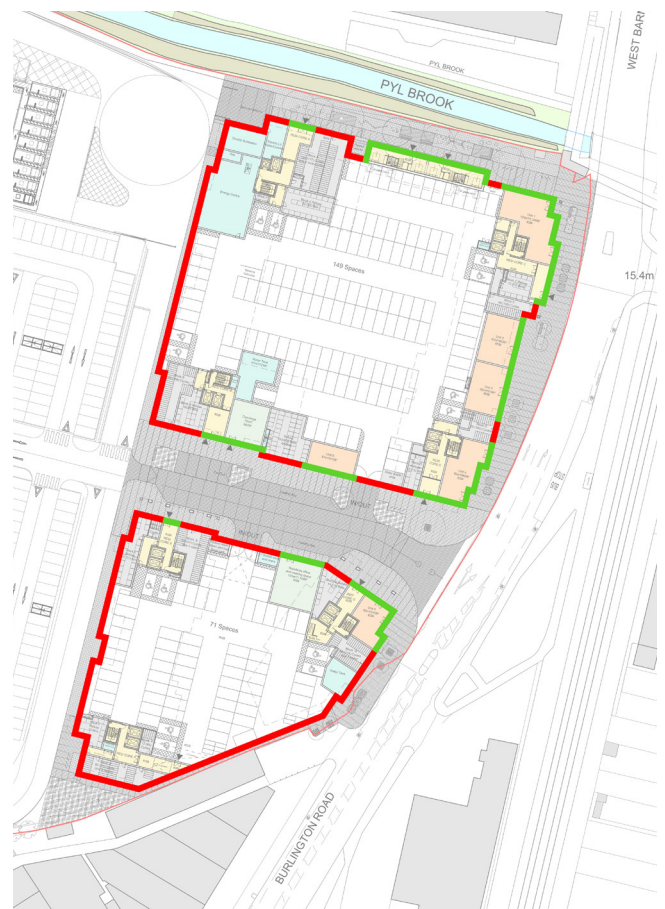
Figure 3.3: Ground floor plan of Appeal proposal (extract from drawing E1180/D6100/P2) marked up to show active frontages (green) and dead frontages (red)
