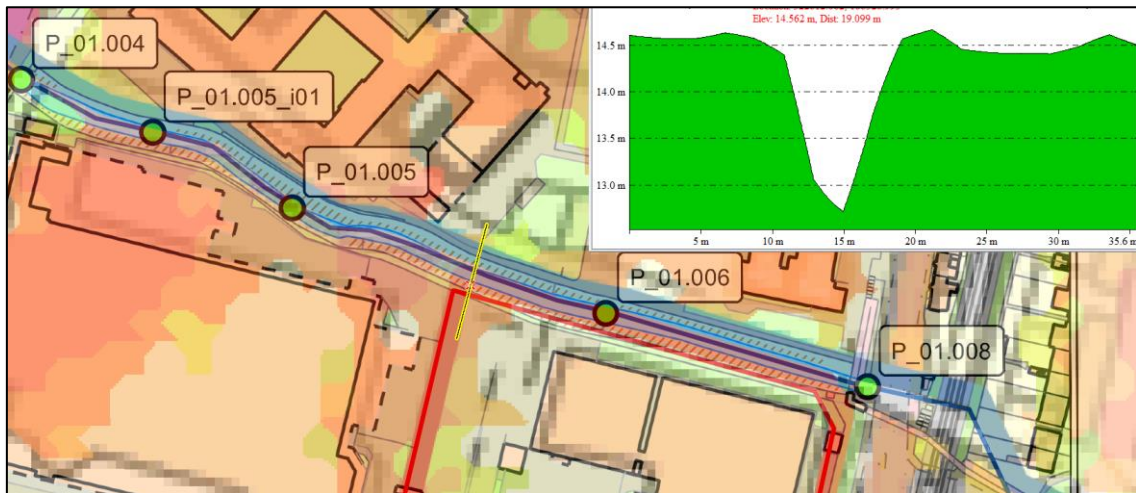
Figure 6 – Transect of river profile, with 1d node location and AEP exceedance demonstrating exceedance of channel
