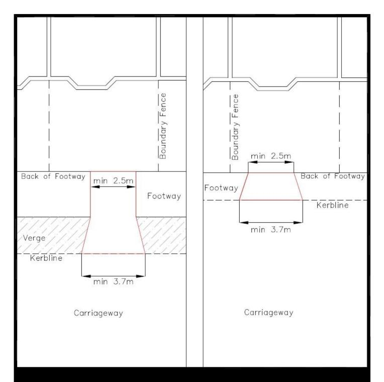
There must be a minimum of 2.5m clear footway width to the back of the footway adjacent to the location of the crossover
