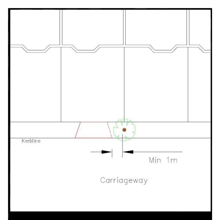
The policy of the Council is to refuse an application for a vehicle crossing if the application would involve the removal of a Highway tree. There must be a minimum of 1.0 metre from the base of the tree to the top of the ramped kerb of the proposed crossover.
