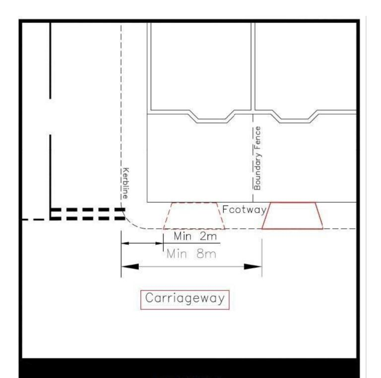
The distance from any junction from the nearest edge of the proposed crossover must be at least 8m (the optimum is 10m). (Refer to Diagram 3). On Cul-de-sacs or permanent No Through roads with less than 30 properties a minimum of 2.0m from the kerb line may be considered.
