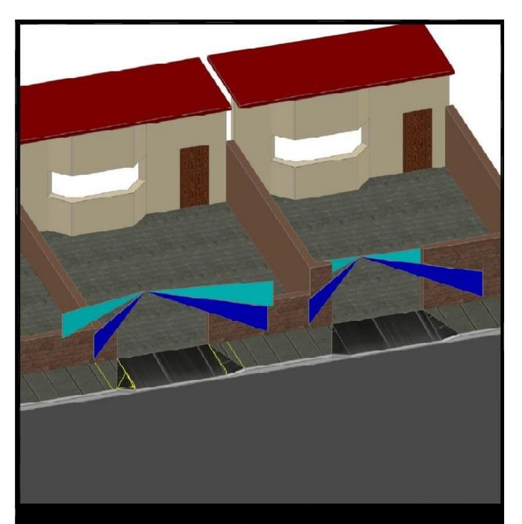
This measurement is used to ensure any hedges or walls marking the property boundary would not obscure pedestrians using the footway from the vision of the driver of an exiting vehicle. (1.5 metres inside the property line from the centre of the proposed crossover.)
