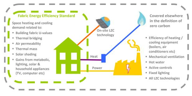
Figure iii: Task Group definition of the scope of the Fabric Energy Efficiency Standard
