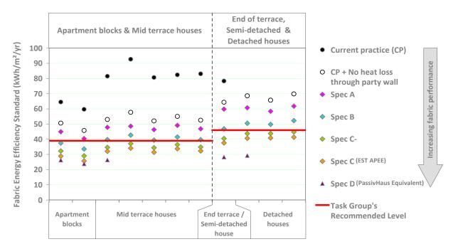
Figure v: Recommended level of the Standard shown with the range of specifications modelled
