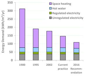
Figure xii: Energy demand of a semi-detached home built to different building standards, assuming contemporary comfort levels, hot water usage and appliance use
