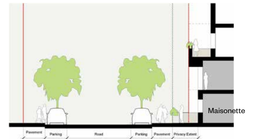
Section BB: Indicative section of ground floor maisonette potential interface with street
