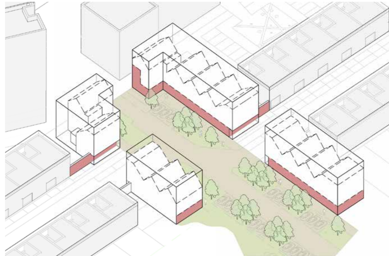
Housing Court - Illustrative birds eye view showing the continuous plinth at ground floor level
