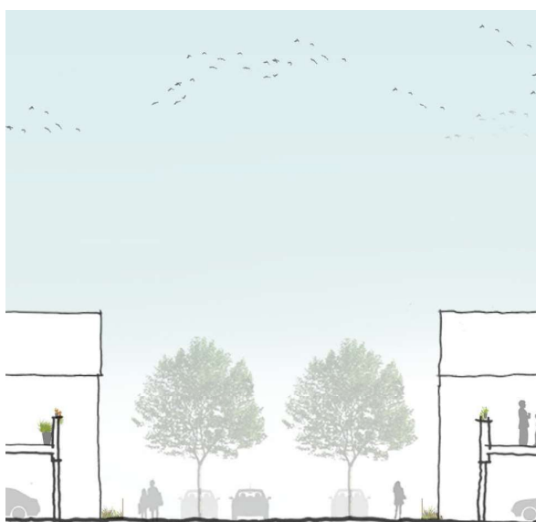
On plot parking Foot path Parallel parking Carriage way Parallel parking Foot path On plot parking
