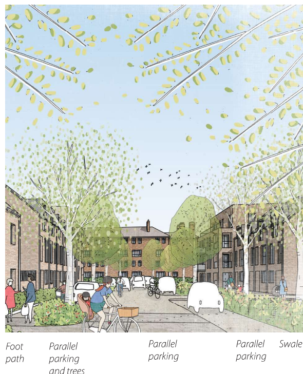
Indicative illustration of secondary street with swale
