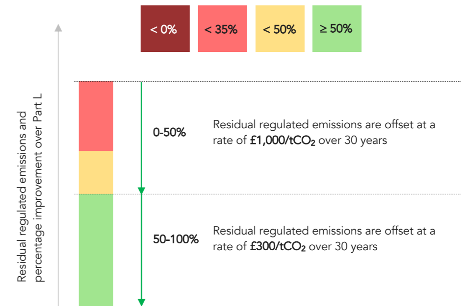
Figure 2 - Recommended tiered carbon prices for non-domestic buildings . There is no third tier due to the limitations of Part L/SBEM for non-domestic buildings which make it more challenging to achieve an 80% improvement for all typologies.
