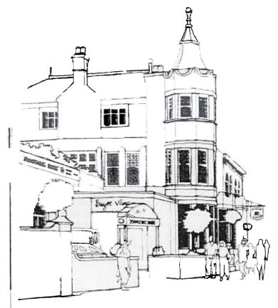
The corner element has a symmetrical, arched, Victorian entrance insert at ground level and semi circular headed timber vertical sliding sashes at first floor which repeat on the return elevation. The return ground floor has fixed casements over a dado height glazed tile plinth which extends across the adjoining three storey element. This element also has recessed timber vertical sliding sashes in four panes on its upper floors.
